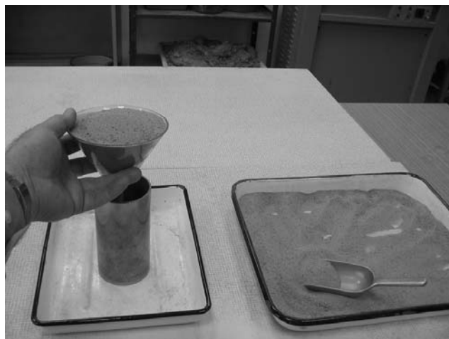
Fig. 1. Test procedure: a) \rho_{dmin} , b) \rho_{dmax} according to PN-88/B-04481 [15].
